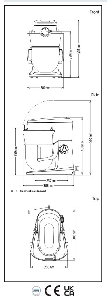
Electric Supply voltage: 200-240 V/1N ph/50/60 Hz **Total Watts:** 0.5 kW Capacity:
